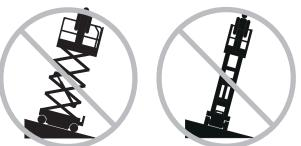
Do not depend on the tilt alarm as a level indicator. The tilt alarm sounds on the chassis only when the machine is on a slope.
